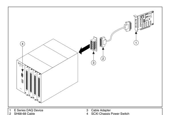
Figure 1-3. Connecting an SCXI Chassis to an E Series DAQ Device
