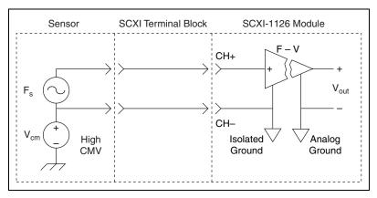
**Figure 2-1.** Ground-Referenced Signal Connection for the SCXI-1126 with High Common-Mode Voltage
